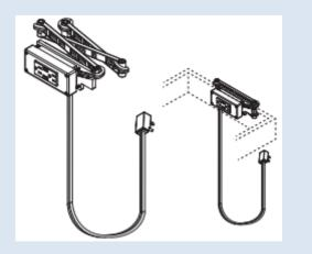
This modification installs a compact drawer outlet into the drawer box. Includes two 120V electrical plug-ins and two 2.1 amp USB charging ports. Available on base cabinet widths of 18"-36" and depths of 15", 18", 21", and 24". Installs in left drawer (**DRWPWRL**), right drawer (**DRWPWRR**), or both drawers (**DRWPWRB**). Outlet is ETL approved -compliant for electrical and other standards including US and Canadian safety standards.
