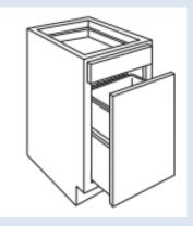
This modification changes the guide mechanism on the wastebasket pull-out to a mechanical push-toopen guide with QuietClose. Available on 24" deep cabinets only. This does not change any other drawer guides on the cabinet.
